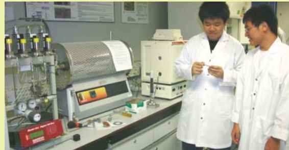
Nanotechnology : Students running the temperature programmed reduction for a nanocatalysis project
