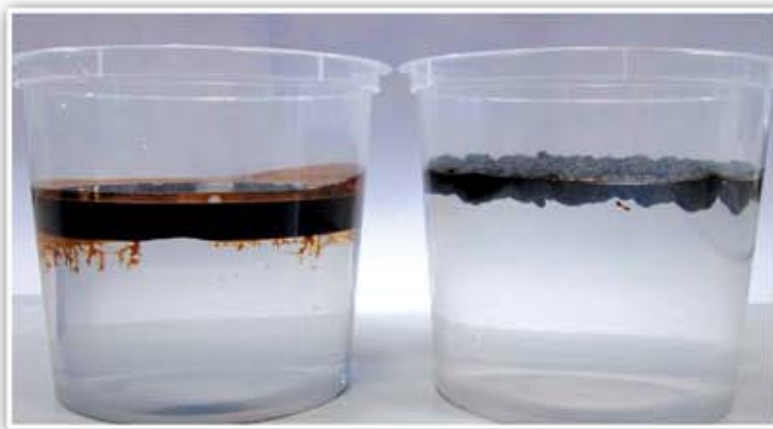
Before/After pictures showing adsorption of crude oil by chitosan-coated carriers
