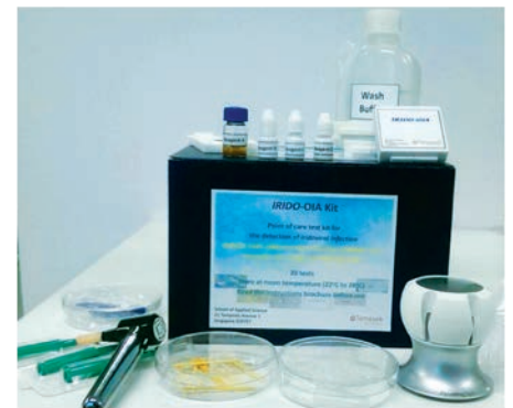
Figure 4: Iridovirus-OIA kit with sample extraction gadgets and test device
