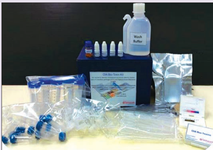
Figure 1: Components of the OIA biotoxin detection kit
