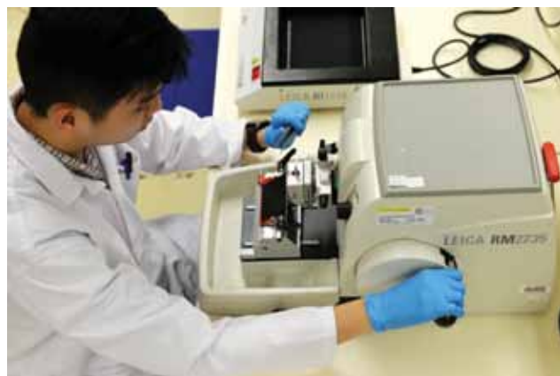
Cutting 4-5 \mu\text{m} sections of paraffin-embedded tissues using a microtome
