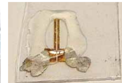
Carbon Nanotube Field Effect Transistor (Crucial part of the developed gas sensor)
