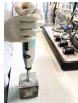
Rebound hammer test on ECC
