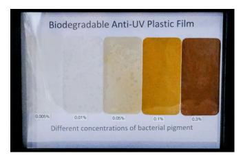
Made from naturally occurring compounds, this biodegradable bioplastic is also non-toxic. Containing a bacterial pigment, the bioplastic has the capacity to absorb blue light and ultraviolet (UV) radiation. The film can potentially replace harmful plastic films, and can also be used to block damaging blue light from computer screens and phones.
